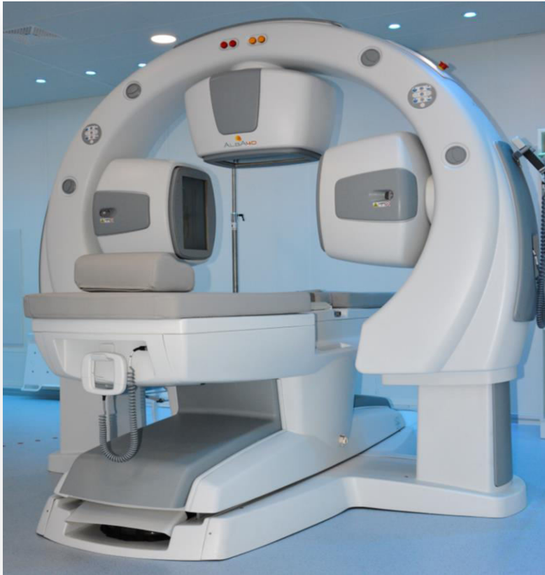
Phased array of 4 antennas emitting at 70 MHz, for deep tumors
